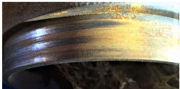
Impeller to wear ring contact
