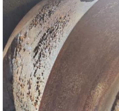
Cavitation damage to impeller vane
