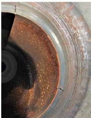
Impeller to suction cover contact
